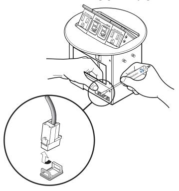
Figure 3-2 — Releasing the bezel plug-in detent (HSA 222 models)
